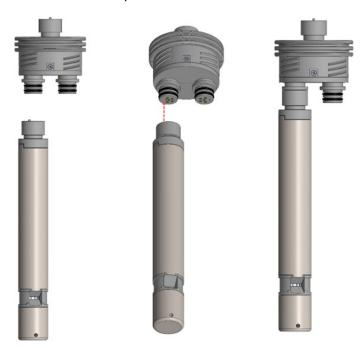
2. Snap the straight collar pieces onto the sensor one at a time, starting with the collar piece that has the fingers, as shown in the following illustration.
