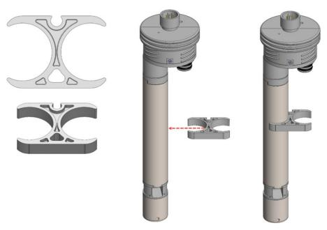
4. Snap the second sensor onto the stabilizer. Then slide the sensor toward the adapter.
